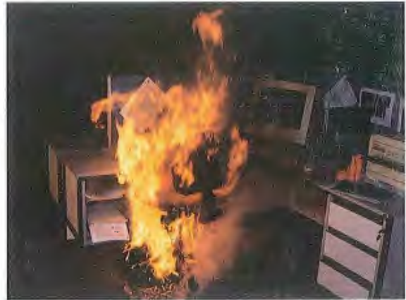
Figure 6: Office fire during early phases of development
