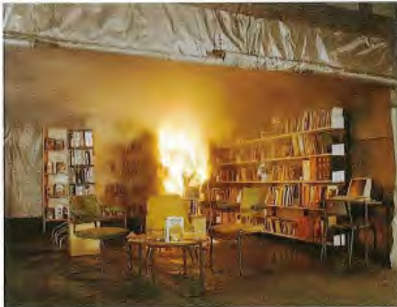
Unsprinklered test after 6 minutes (approximate fire size of 1 MW)
